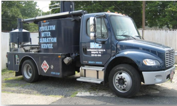
1500 Gallon Prover w/ 100 Gallon Piggyback Can Bottom & Top Load Petroleum Products and Lube Oils
