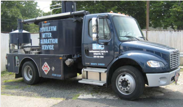
1500 Gallon Prover w/ 100 Gallon Piggyback Can Bottom & Top Load Distillate Petroleum Products and Lube Oils Up to 1000 GPM
