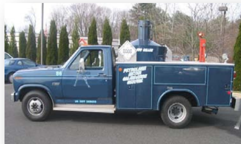
Top Load Distillate Petroleum Products and Lube Oils Up to 200 GPM
